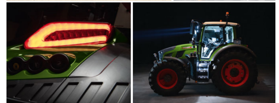
New LED tail lights (CAN-capable) with dynamic sweeping indicator
