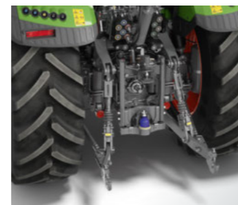
Rear power lift with quick arresters and side support (EU)
